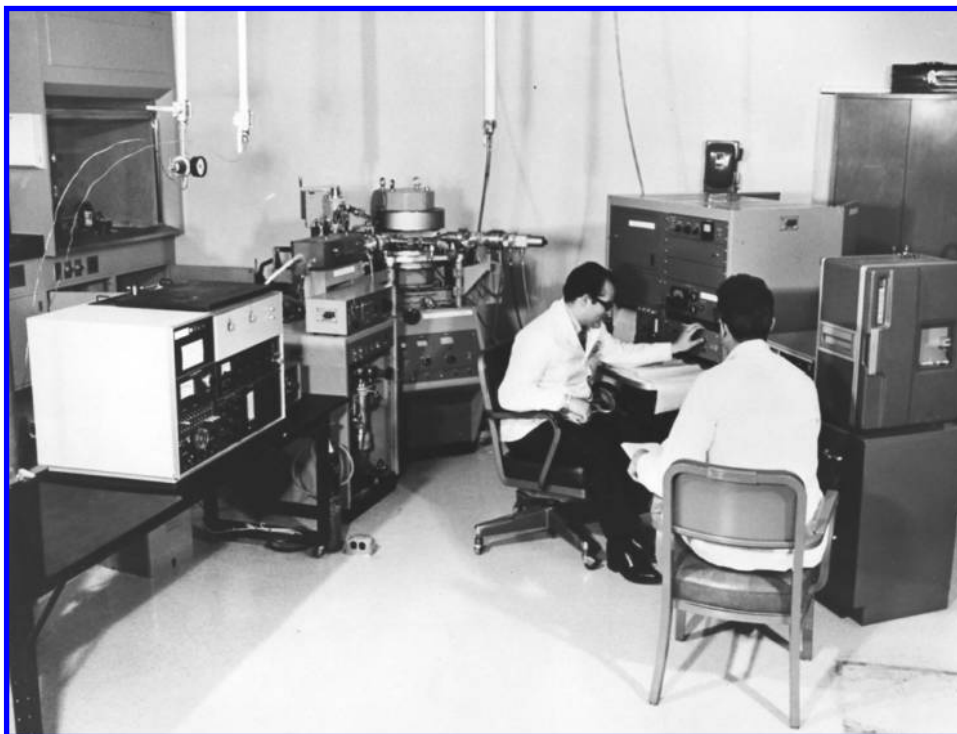
Figure 4. Early Hitachi RMU-6E GC-MS instrument employed to identify volatile compounds in flavors (1969) (courtesy International Flavors & Fragrances).
