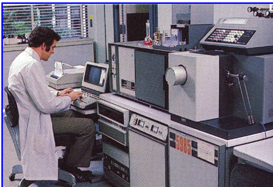
Figure 5. Author using a Hewlett-Packard 5985 GC-MS instrument for identification of dairy flavor volatiles (1982) (courtesy Kraft Foods).
