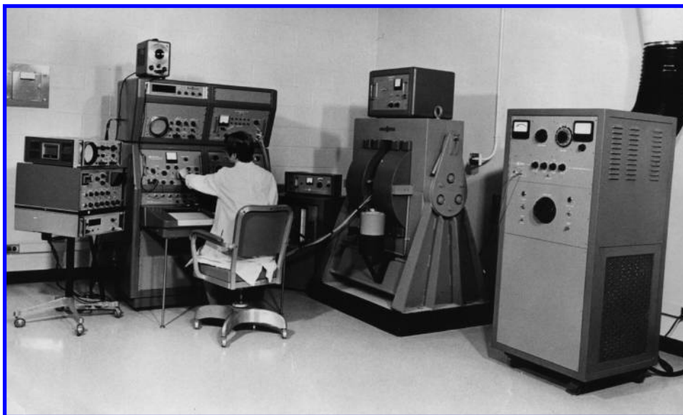
Figure 6. Varian HA-100 (100 MHz) NMR applied for identification of flavor compounds (1968) (courtesy International Flavors & Fragrances).
